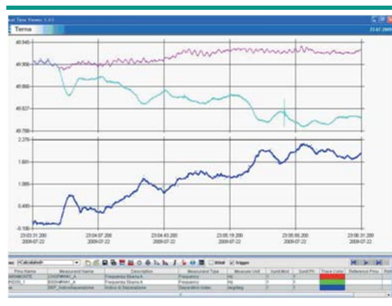
Figure 21: Application of the algorithm for the detection of network separation; the increasing separation index (bottom curve) denotes that the system has split into islands.
