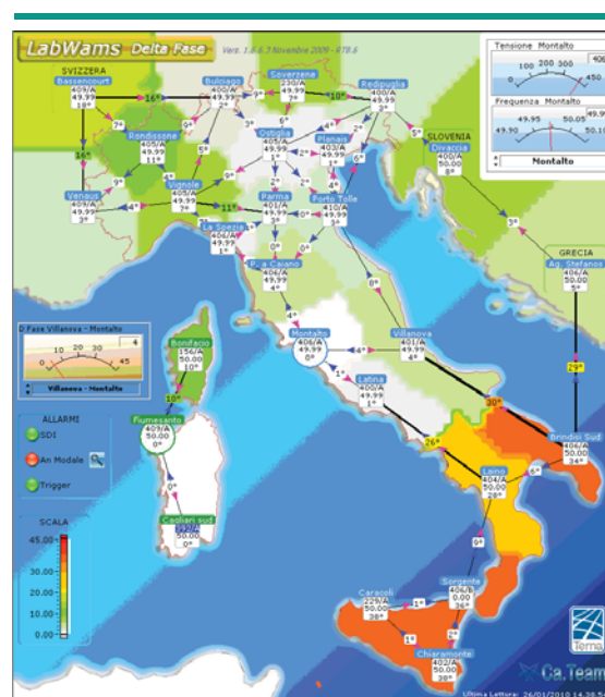
Figure 20: A typical geographic display of the WAMS platform. The background colours of the map depend on the voltage magnitude.
