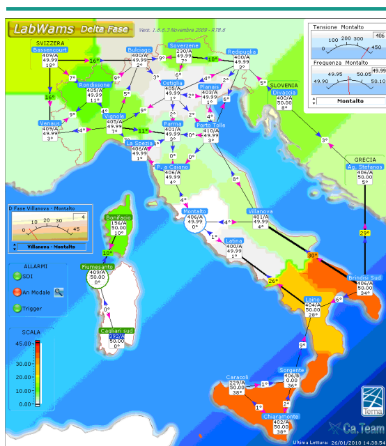
Figure 25: A typical geographic display of the WAMS platform. The background colours of the map depend on the voltage magnitude.
