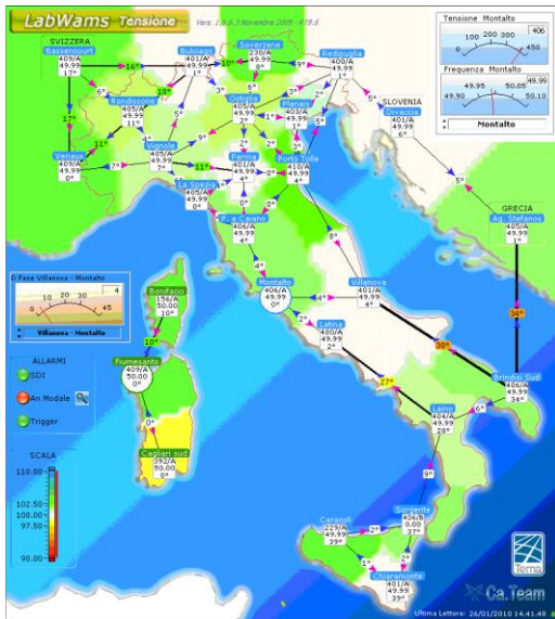
Fig. 5 A typical geographic display of the WAMS platform. The background colors of the map depend on the voltage magnitude
