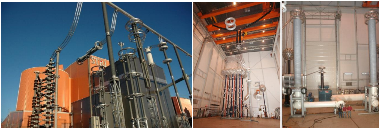
Figure 12 Testing of UHVDC 800 kV for China and India and 1100 kV UHVAC GIS for China (STRI)
