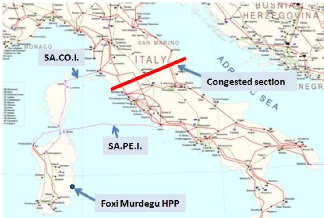
Figure 15 - Italian Electric Transmission Network with Evidence of Sardinian Interconnection (SA.PE.I. and SA.CO.I. Systems) Respect to the Continental Most Congested Section. Position of Foxi Murdegu Hydro Power Plant (Graphical Elaboration of the Original Map, ENTSO-E Properties)
